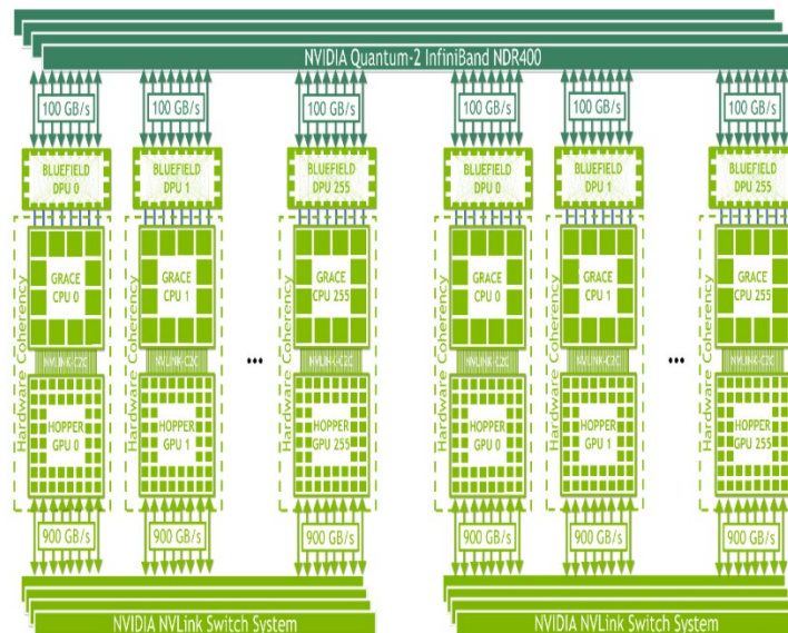
Figure 14. NVIDIA HGX Grace Hopper with NVLink Switch System for strong-scaling giant ML and HPC workloads
