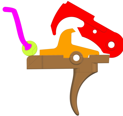
Super Safety Installed, Lever and Cam Rotated
